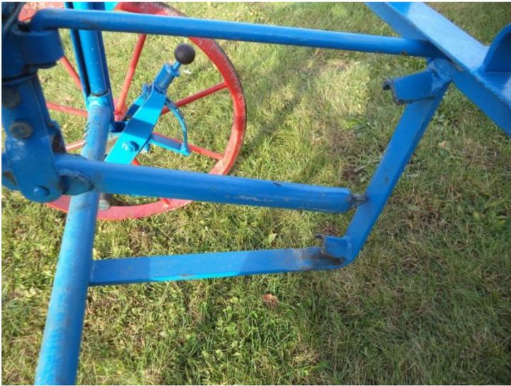
*Image 22: Showing the end of the steer bar, which can be locked in the holder. The holder is the lower triangle in the corner of the frame. The weight of the toolbar pushes it into a locked position (see Image 11 for the transport position).*
