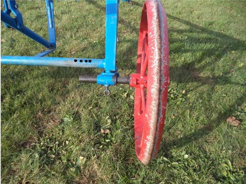
*Image 12: Adjusting the wheel width: the ring bolt can be loosened to move the wheel axle more inward or outward.*
