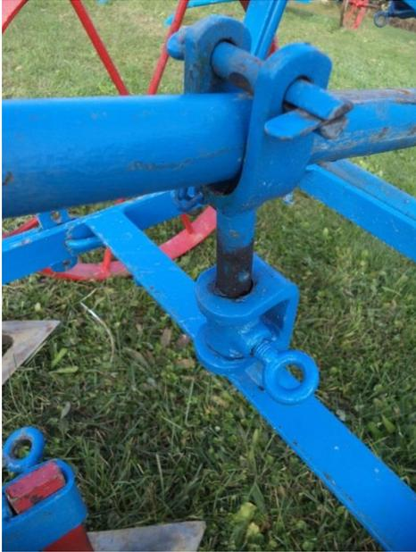
*Image 14: The ring bolt can be loosened so the steering bar can be put higher or lower. The vertical round bar has holes in it where the bolt is screwed into.*
