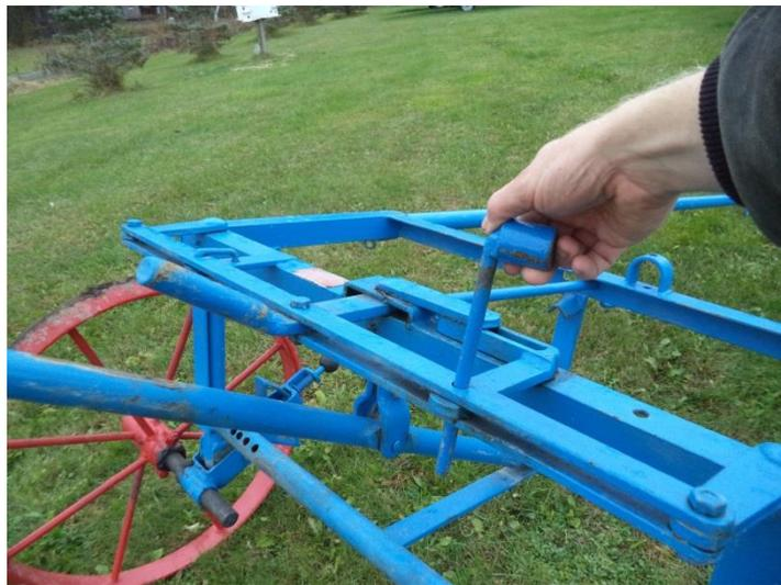
When using the “plant hole makers”, the bicycle part of the steer is put off the machine. The rest of that round bar is used as a lever to lift up and to lower the “plant hole makers”. For either transport or work mode. There another bar is attached to the tool carrier. Which functions as the steer. Then pin shaped hammer is stays in place and the other pin is pulled out. Making it possible to steer the wheels.
