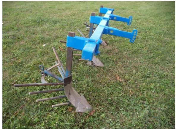
*Images 16 & 17: The disconnected toolbars for quickly changing to from for example: hoeing to hilling.*
