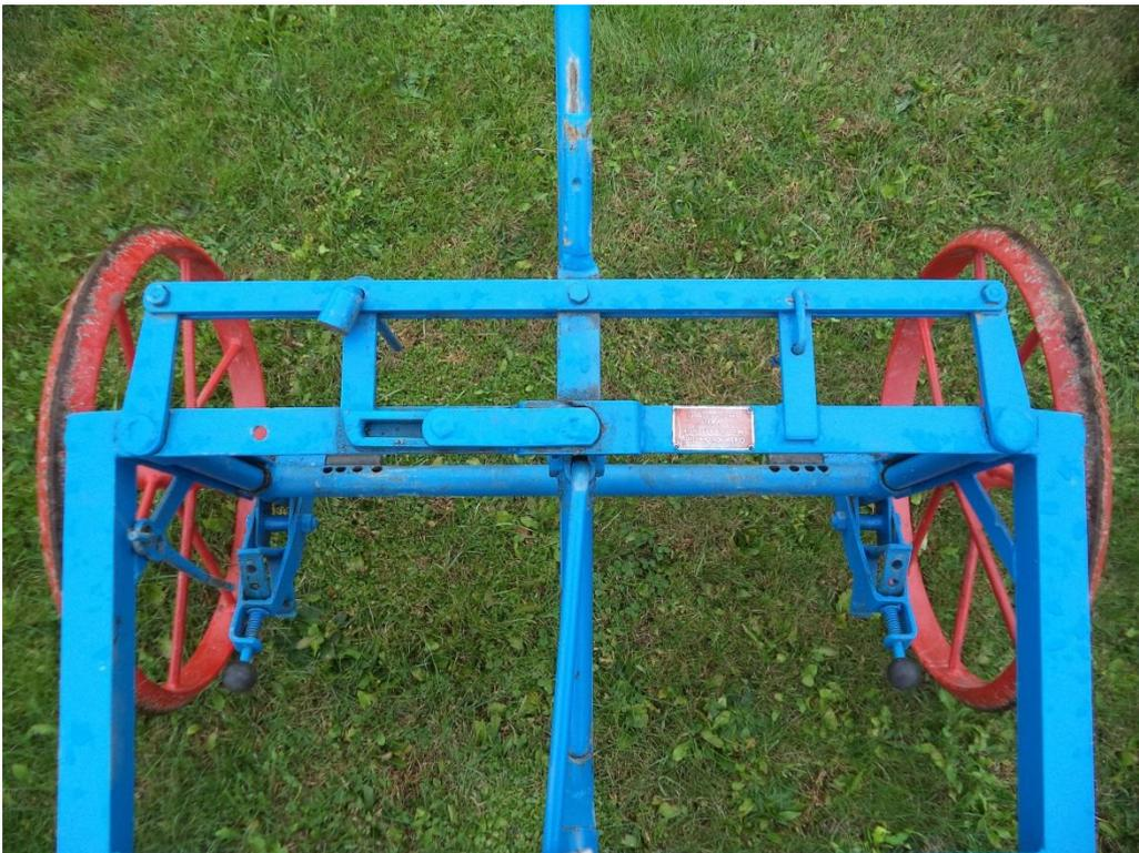
*Image 6: The toolcarrier steering system in transport mode.*
