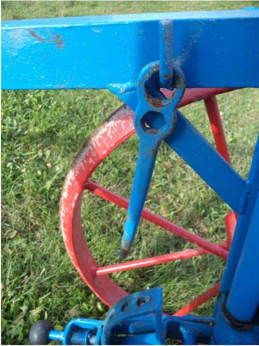
*Image 23: Next to the hammer there is also a wrench. For two sizes and the tail is used for the ring bolts.*
