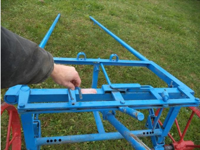
*Image7: When this pin is pulled out, the tool carrier comes out of transport position. Then the toolbar and wheels both become steerable.*
