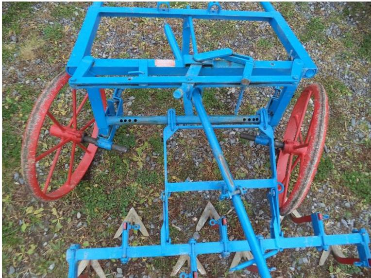
*Image 10: a closer look up to the steerage system when steered to the right with wheels and toolbar.*
