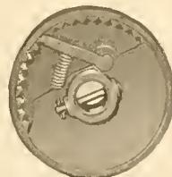
Clutch. Part of casting has been cut away to show construction of pawl and ratchet. It can be disengaged when machine is not operating
