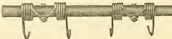
Showing manner in which teeth are fastened to the tooth bar
