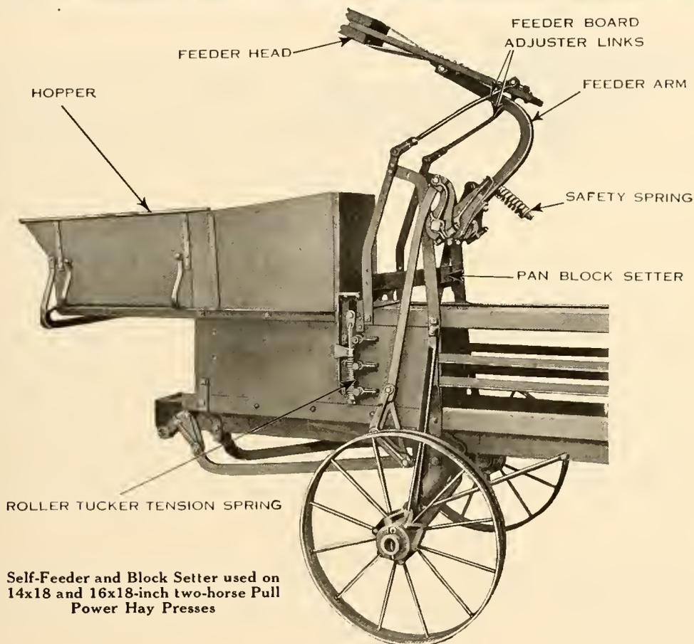
Self-Feeder and Block Setter used on
