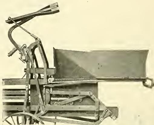
Toggle Joint Plunger, end of stroke,
