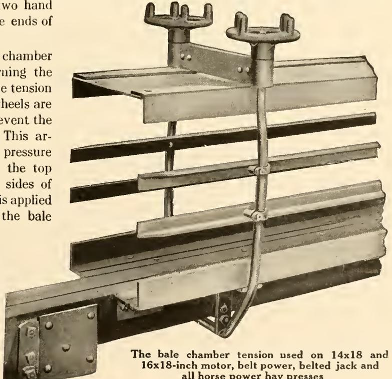
The bale chamber tension used on 14x18 and 16x18-inch motor, belt power, belted jack and all horse power hay presses
