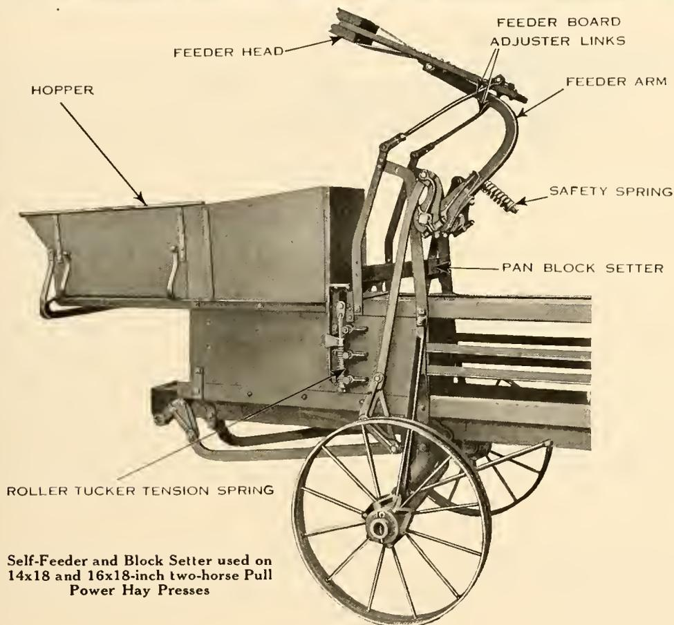
Self-Feeder and Block Setter used on
