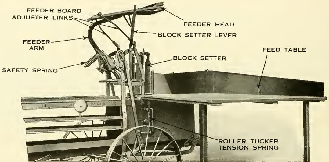
Showing rear end of International Motor Hay Press with 17x22-inch bale chamber.
