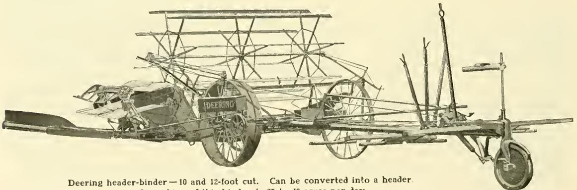
Deering header-binder—10 and 12-foot cut. Can be converted into a header.
