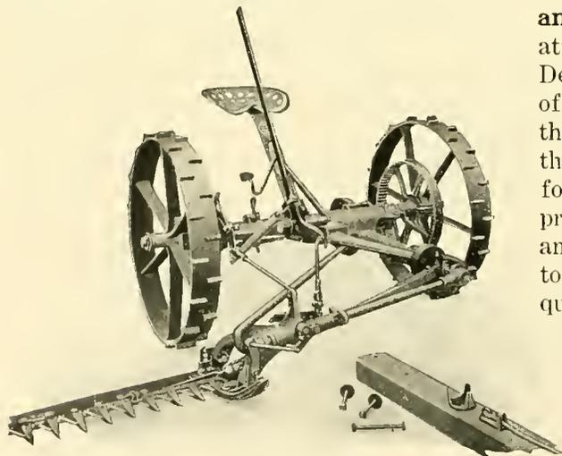
Tongue can be taken out by removing three bolts and without disturbing the lifting lever mechanism
