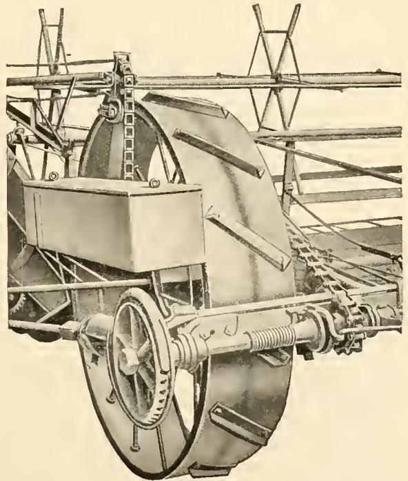
Main wheel and main gear on header-binder
