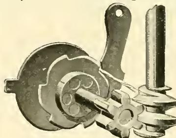
Steel twine-holding disk and pinion
