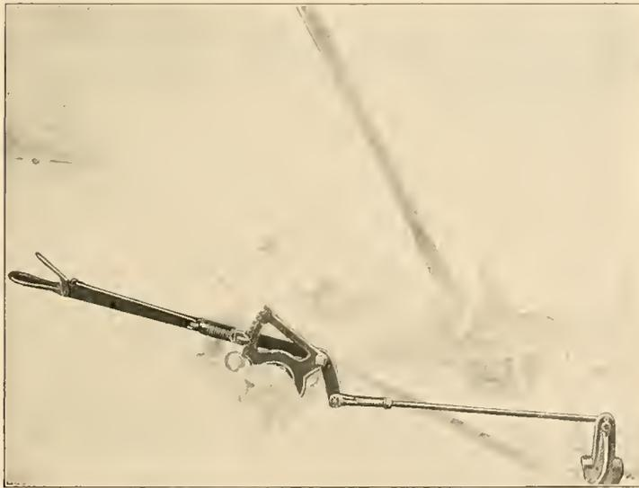
Showing tilting lever, quadrant and connections
