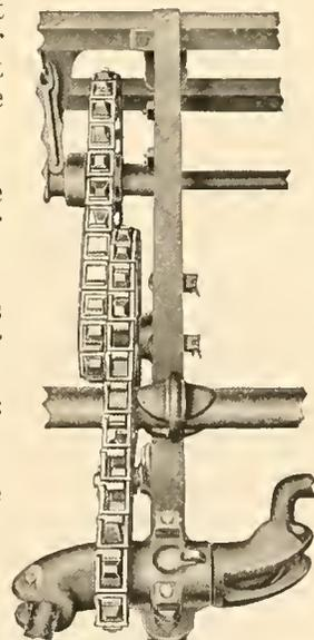
The chain drive is of a practical design and is located in the center of the frame
