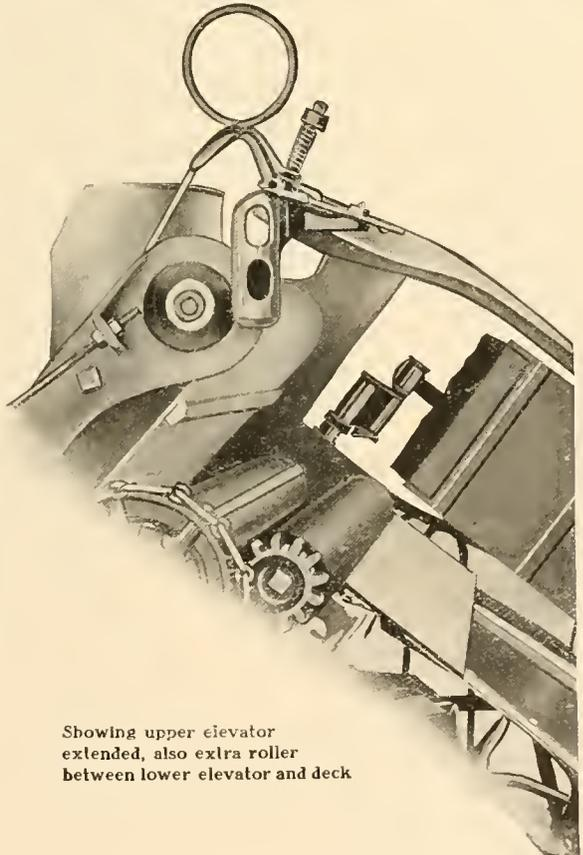
Showing upper elevator extended, also extra roller between lower elevator and deck
