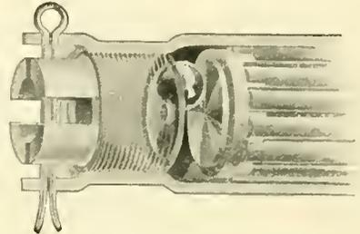
Ball bearing on end of crank shaft
