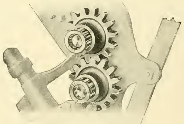
Elevator bearings partly exposed to show rollers
