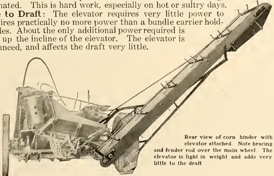
Rear view of corn binder with elevator attached. Note bracing and fender rod over the main wheel. The elevator is light in weight and adds very little to the draft
