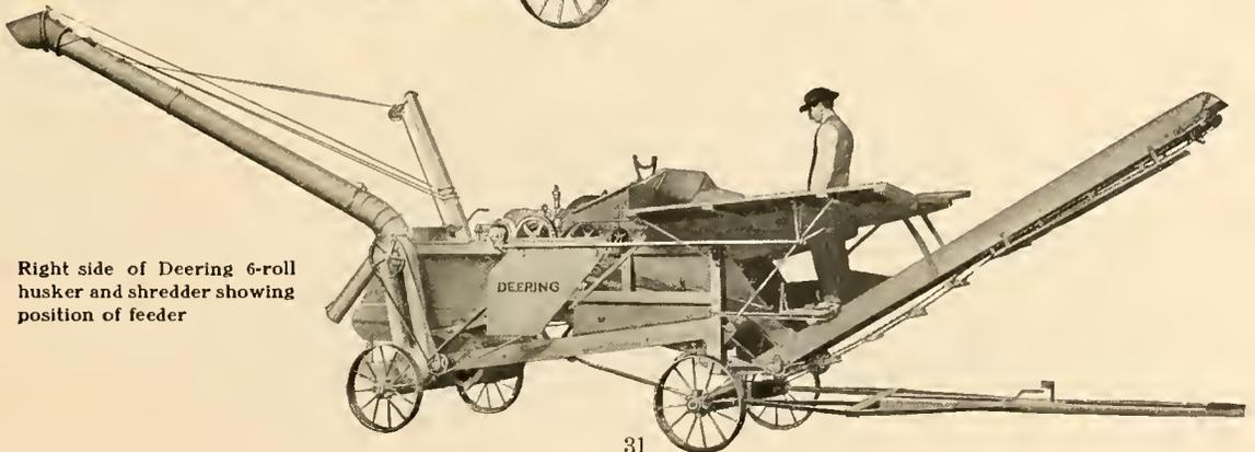
Right side of Deering 6-roll husker and shredder showing position of feeder
